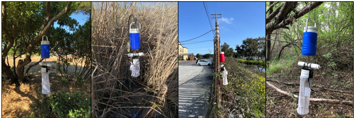
The District laboratory and operations staff set overnight CO 2 -baited adult mosquito traps in a wide variety of ecosystems and neighborhoods. The goal is to capture a representative snapshot of mosquito activity across San Mateo County.
