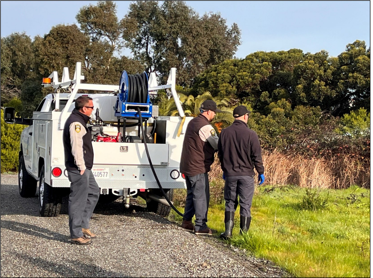
Figure 5- District staff using the new 300-gallon fire hose spray skid to control juvenile mosquitoes in Mills Field. The skid can now fit in the back of a truck which allows for treatment of areas inaccessible with a trailer.
