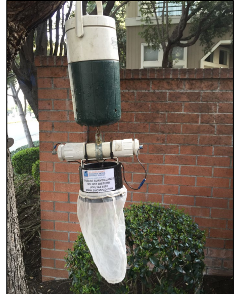
The District uses CO 2 traps to collect mosquitoes for WNV surveillance throughout San Mateo County.
